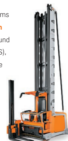
NXV The very narrow aisle truck is the ideal partner for efficient use of space in small warehouses. Optional positioning aids, such as the cross-line laser between the forks or camera systems, help you to position the load accurately.
