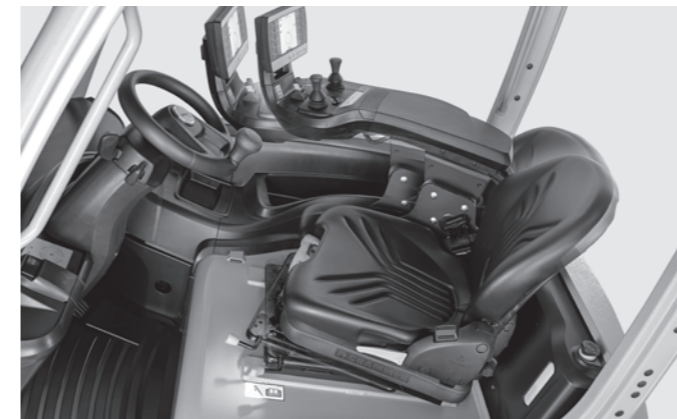
Swivel seat for comfortable reversing
