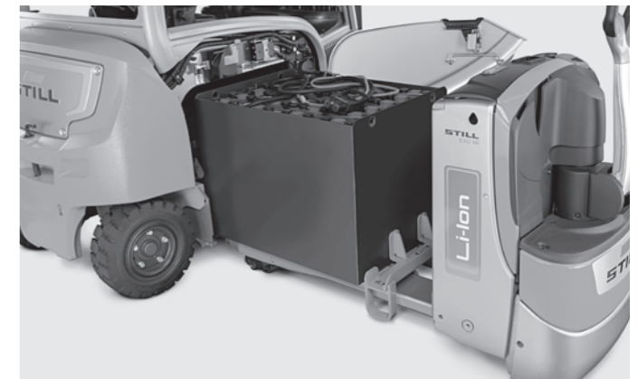
Battery change with electric pallet truck
