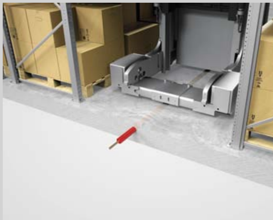
Inductive guidance (guide wire on the ground)
