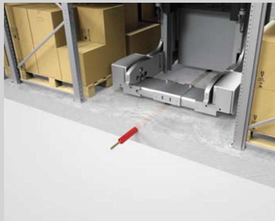
Inductive guidance (guide wire on the ground)
