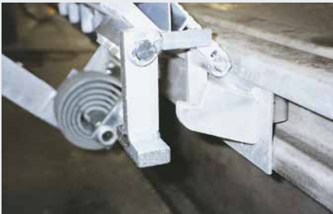
Safety latch locks automatically after vertical positioning.
