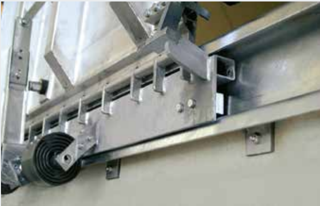
Steel plates 80 x 80 x10 fixed underneath the guide rail or stationary dock leveller.
