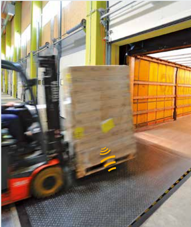
Automatic recording of goods movements, simply while crossing the dock leveller.
